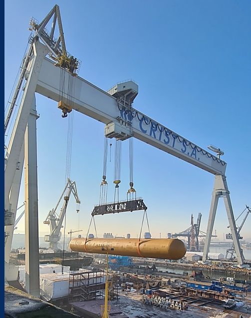
GANTRY Cranes Lifting capacity: 1000 t Span: 153 m Height: 106 m
