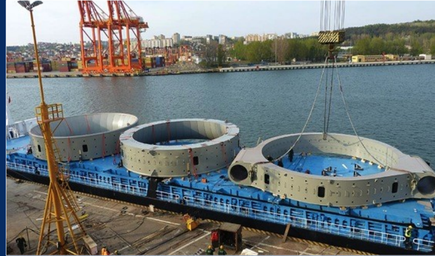
TIDIAL TURBINE End-caps – Outer End-caps each 55 ton
