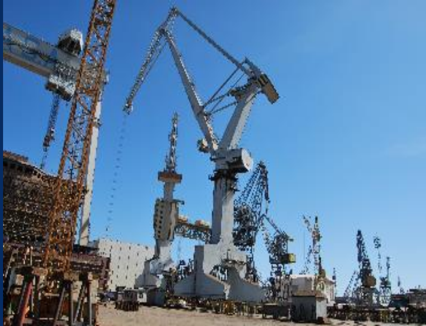
KONE Cranes Lifting capacity: Each of 150 tons
